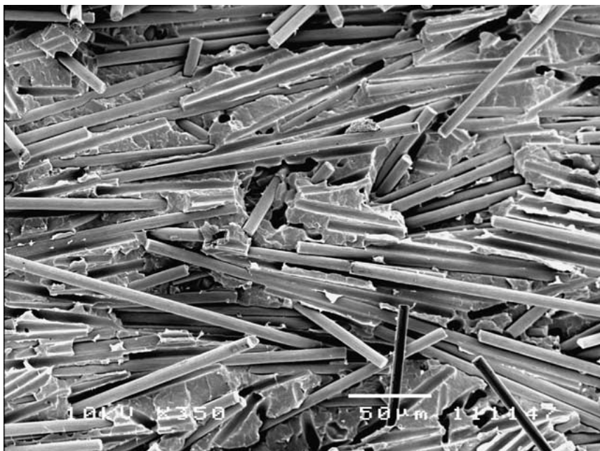
Figure 9 Brittle fracture of the matrix in the core layer for the SCF/PP composite with V_f = 25\% .
